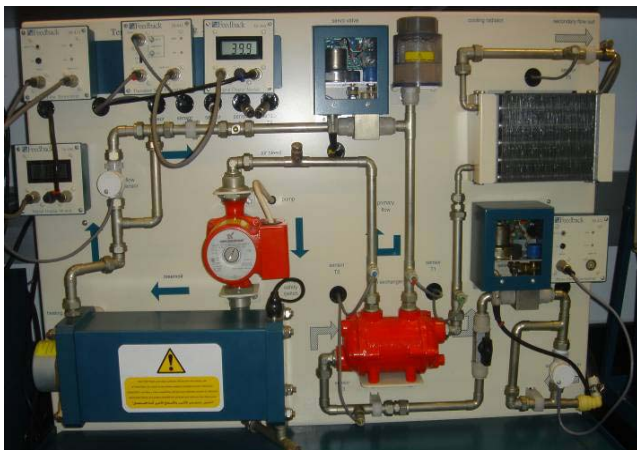
Fig. 2. Temperature Process Control Rig. Students apply feedback control principles to control the primary and secondary flow rates through a heat exchanger.
