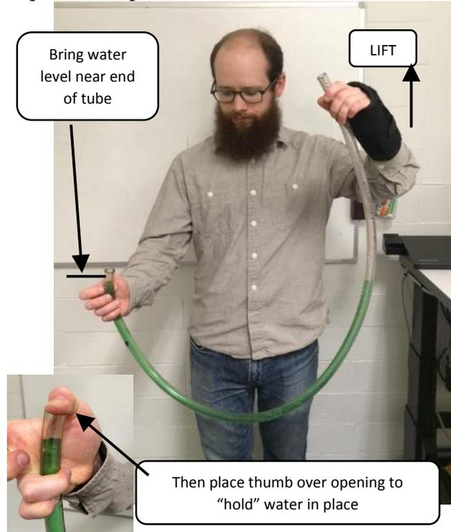
*Figure 10: Shifting the water to one end of the tube*
