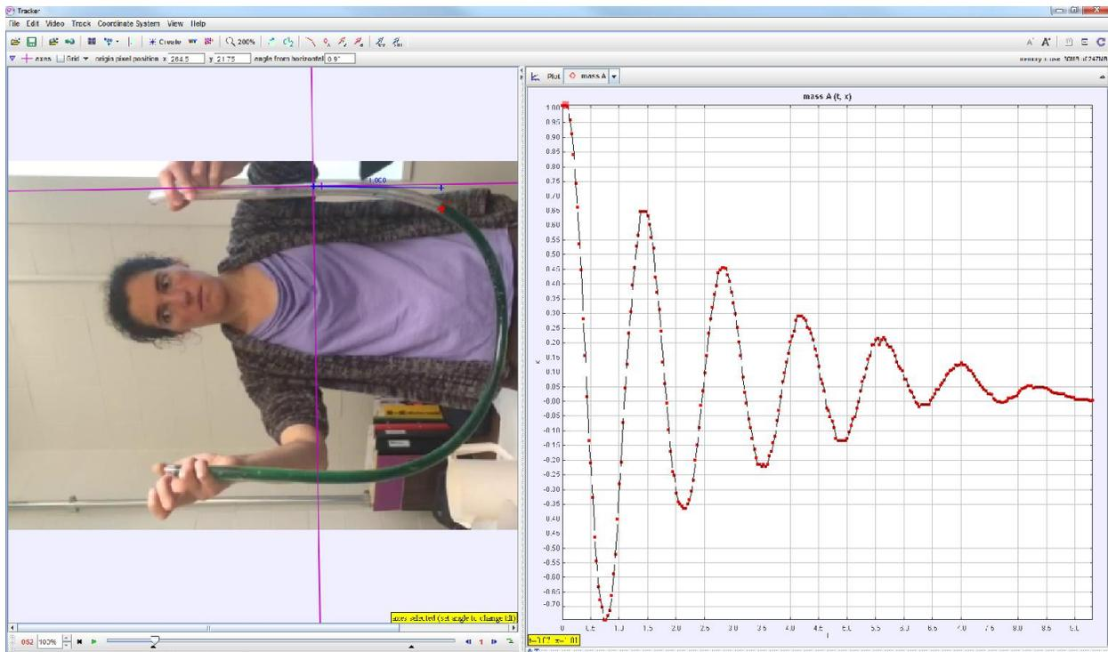
Figure 14: Response when the tube end is fully open demonstrates a low damping ratio
