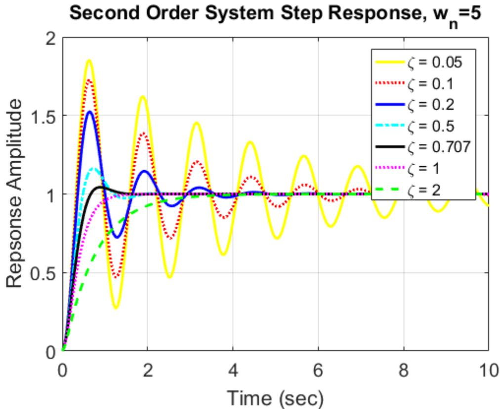
Figure 16: Second order system step response for a range of damping ratios
