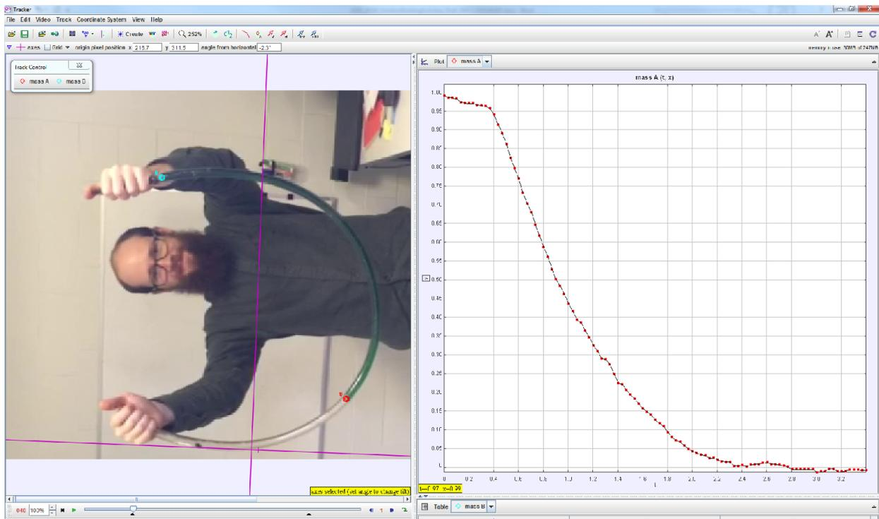
Figure 15: Response with just a pinhole opening at tube end shows a high damping ratio
