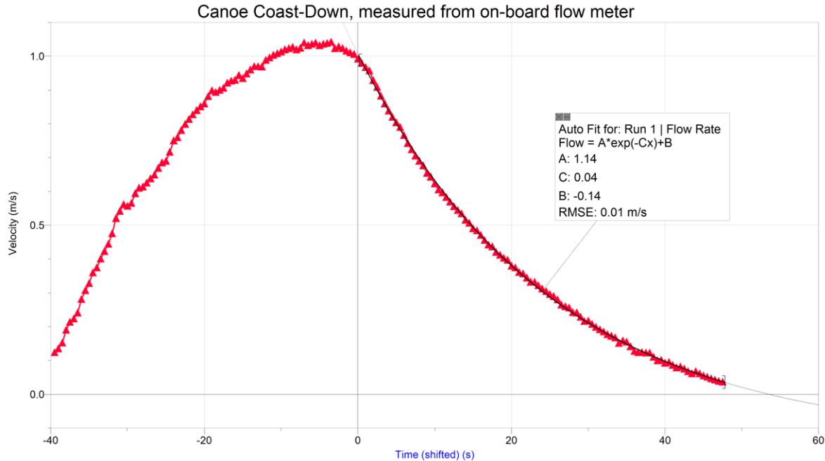
Figure 4: Canoe Coast-down starts at time 0. Data collected from onboard flowmeter. Exponential curve fit displayed as black line.
