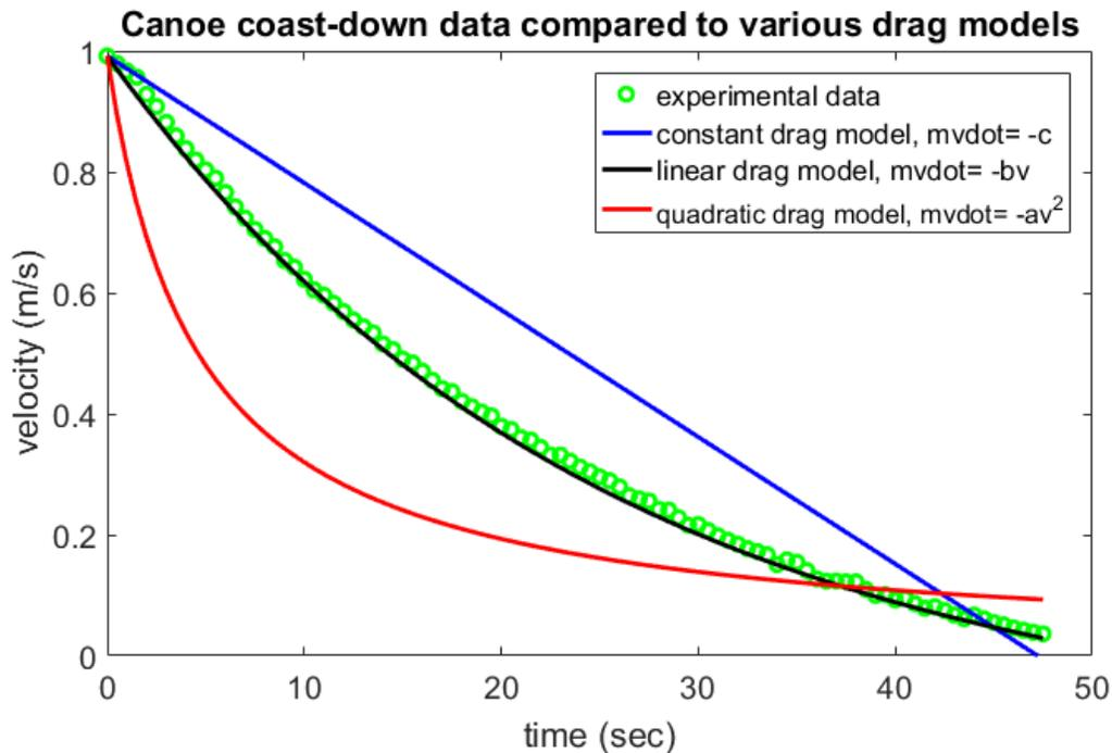
Figure 5: Canoe Coast-down data compared to various drag models
