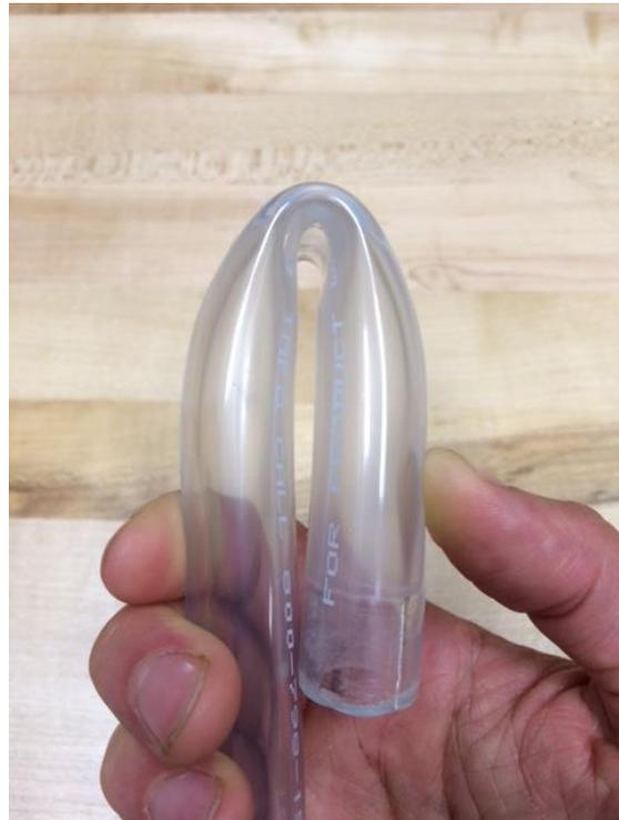
Figure 11: Creating the initial condition      Figure 12: To restrict airflow fold over the tube
