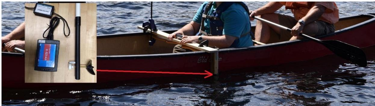
*Figure 3: Flow meter mounting for data collection*
