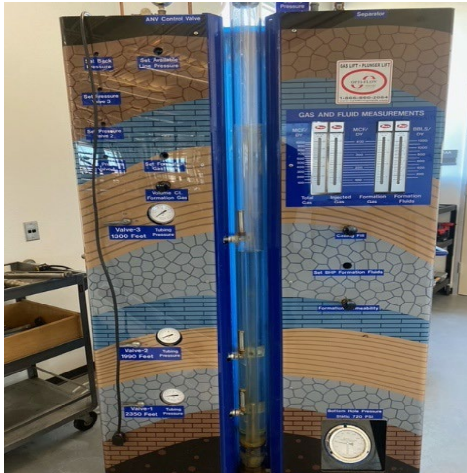
Figure 5 shows a model represents the gas lift technique
