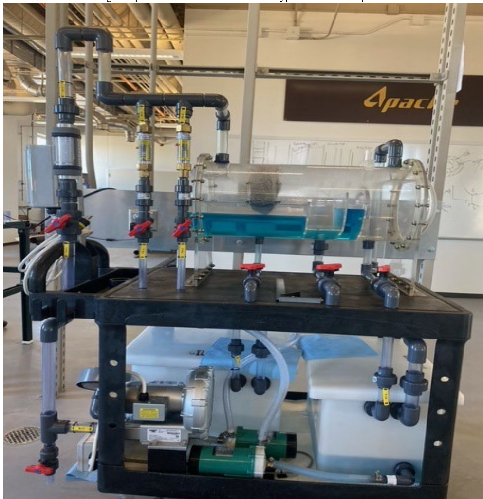
Figure 9 represent a fully functional lab-scale model of a horizontal separator
