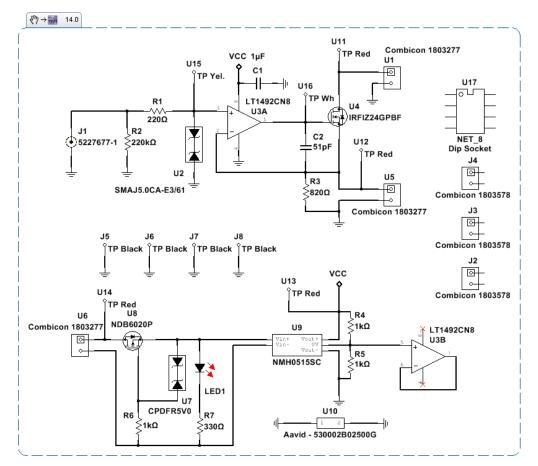
**Figure 9 Supply Transient Tester**
