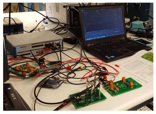
Figure 8 Complete transient load testing bench setup
