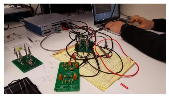
Figure 1 Switching Regulator Laboratory Bench Setup
