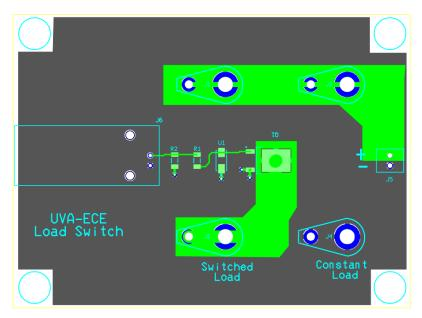
Figure 7 Overlay of Transient Load Switch Printed Circuit
