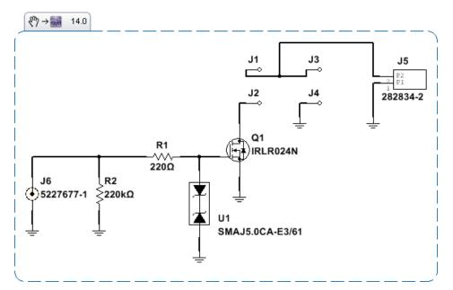
Figure 6 Transient Load Switch Schematic
