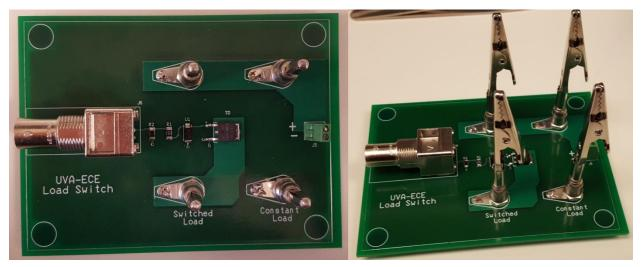
Figure 5 Transient Load Switch
