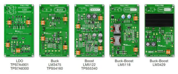
Figure 2 Voltage Regulator Kits (From svnq001.pdf available at ti.com)
