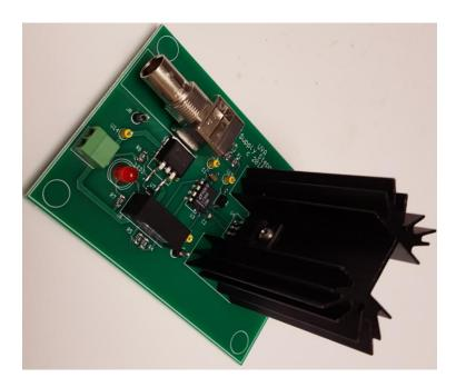
Figure 11 Supply transient voltage tester
