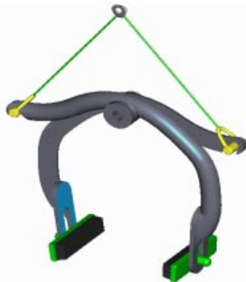
Figure 2. Brake Assembly created during Lesson 8. Use of Skeleton and Assembly techniques.
