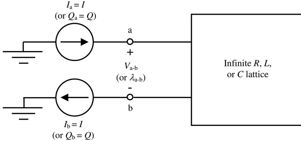
Fig. 3. Test circuit used to calculate  $R_{\text{eff}}, L_{\text{eff}},$  or  $C_{\text{eff}}$
