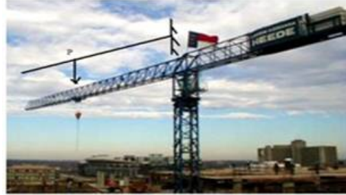
Figure 2. Tower crane overhang as a cantilever beam
