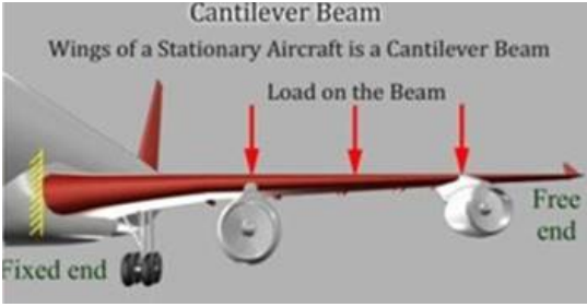
Figure 1. Aircraft wing as a cantilever beam
