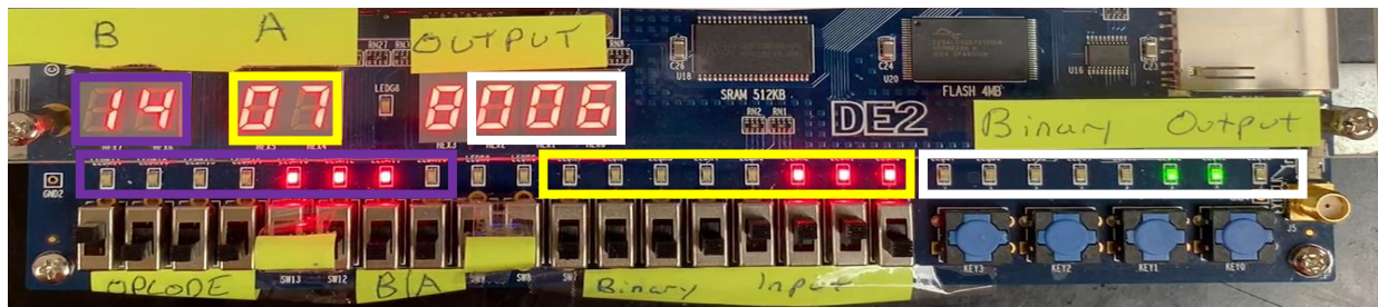
Fig. 1. Input and output in DE2 FPGA board.
