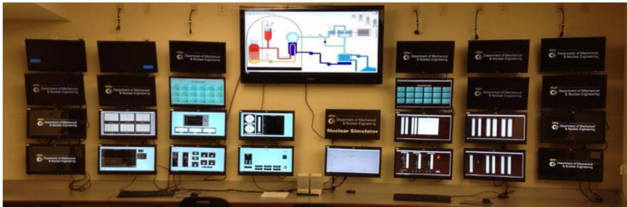
Figure 5: Year two of the nuclear simulator built for safety training and educational purposes. This project continues to be used for demonstrations during school visits.
