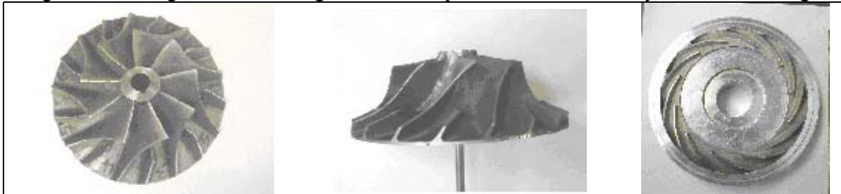
Figure 2A. From left to right: top view of impeller, side view of impeller, vaneless and vaned diffusers.
