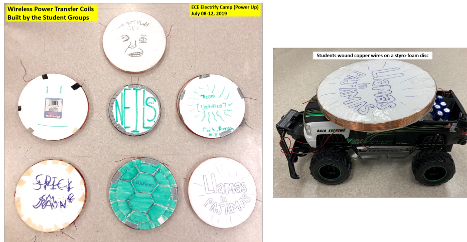
Fig. 2. Receiver coils made by different student groups. Some student groups selected different radii and also had different number of turns.
