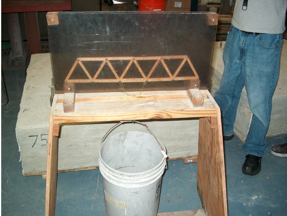
Figure 1. Typical student truss bridge with large craft sticks in testing frame
