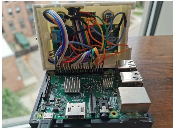
Fig. 7. The prototype Control Panel's inner wiring
