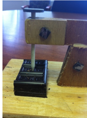
Figure 3. The chocolate hardness tester with a sample of dark chocolate is shown. The “weight” attached to the top of the indenter is a roll of pennies.
