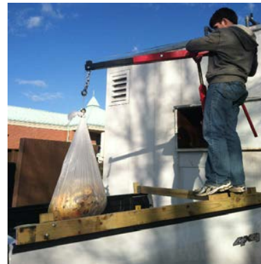
Figure 8: The first iteration design to load waste into the digester used a jib crane. Subsequent student efforts have re-designed this system
