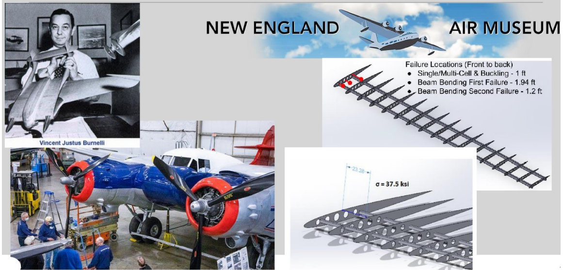
Figure 5: Structural analyses of the wings completed by one groups working on the Burnelli CBY-3, provided by the New England Air Museum during 2022-2023
