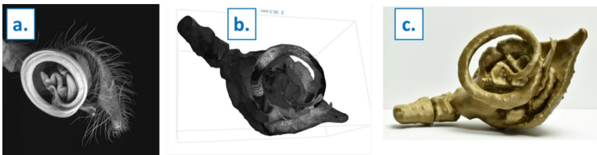
Figure 9. Inner surface view of a spider pedipalp showing SEM image, 3D CAD representation, and enlarged 3D printed model.
