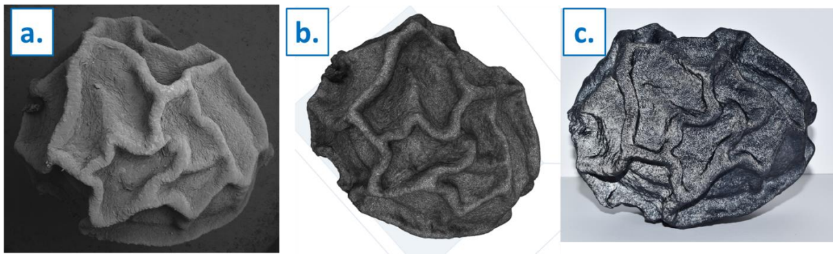
Figure 6 SEM image, 3D CAD representation, and scaled 3D printed model of a black peppercorn.
