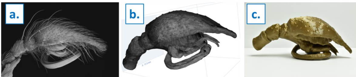
Figure 8. Side view of a spider pedipalp showing SEM image, 3D CAD representation, and enlarged 3D printed model.
