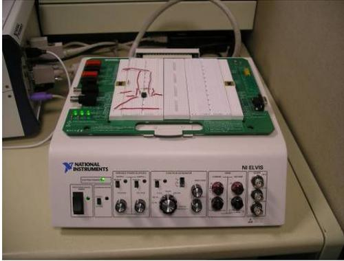
Figure 2: The National Instruments ELVIS electronics workbench.
