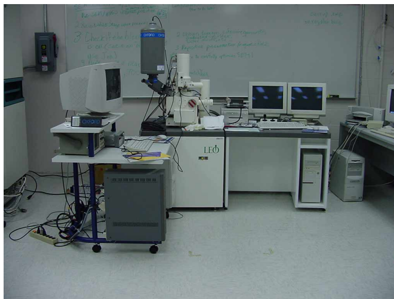
Figure 1. LEO 1430 VP Scanning Electron Microscope System with nanoscale imaging, analysis, and patterning capability
