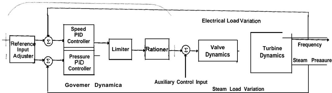
Figure 2. Block Diagram of a cogeneration plant.
