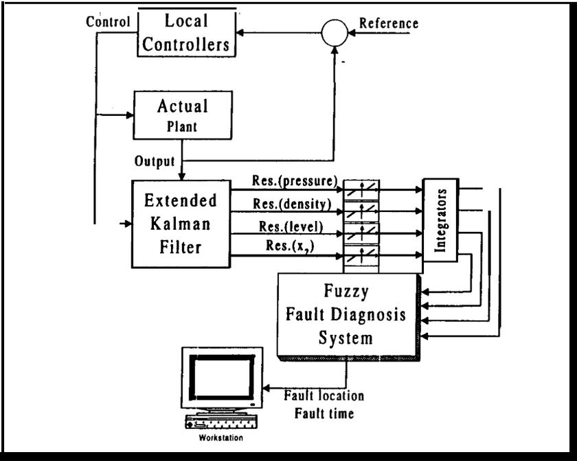
Figure 6. Functional block diagram for fault diagnosis.
