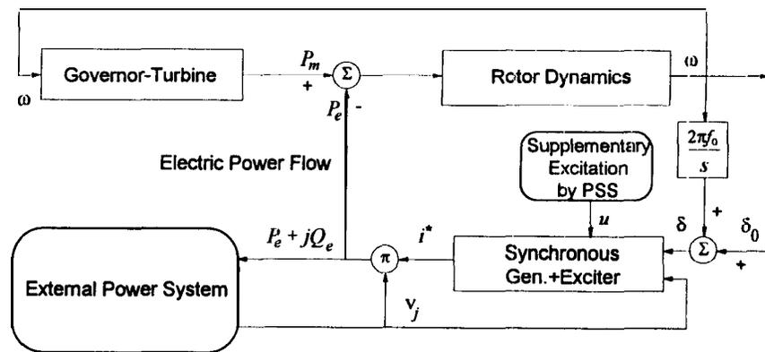
Figure 5. A generator connected to a power system network.
