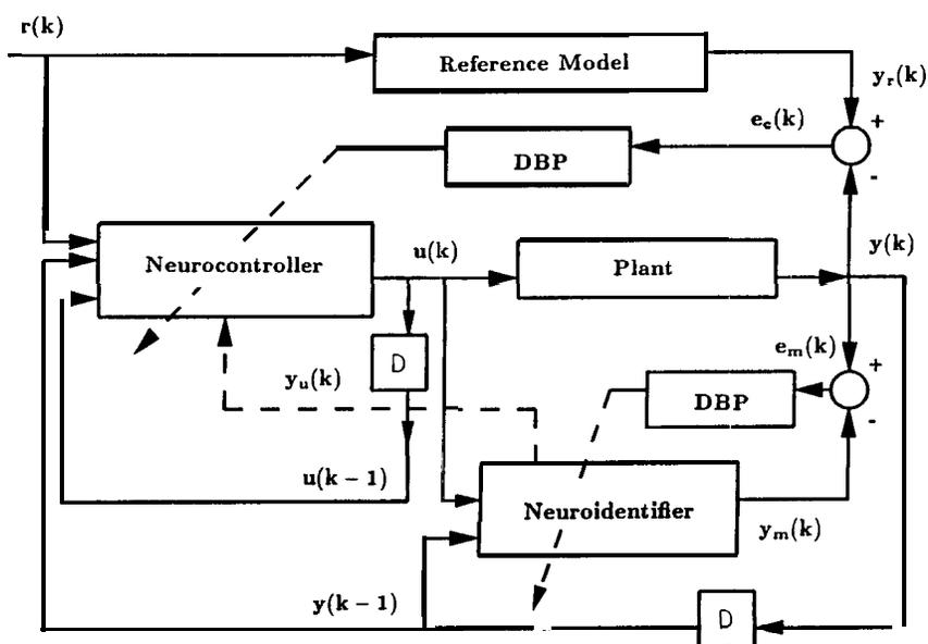
Figure 4. Block diagram of DRNN based control System,
