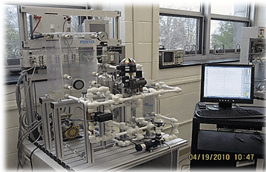
Figure 6. Remote controlled Hydraulic plant experiment controlled with PLC at our department.
