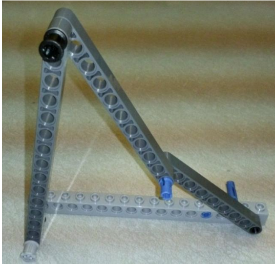
Figure 2, a system for constructing four bar pin jointed mechanism adopted by another group of students from Lego Mindstorm parts.
