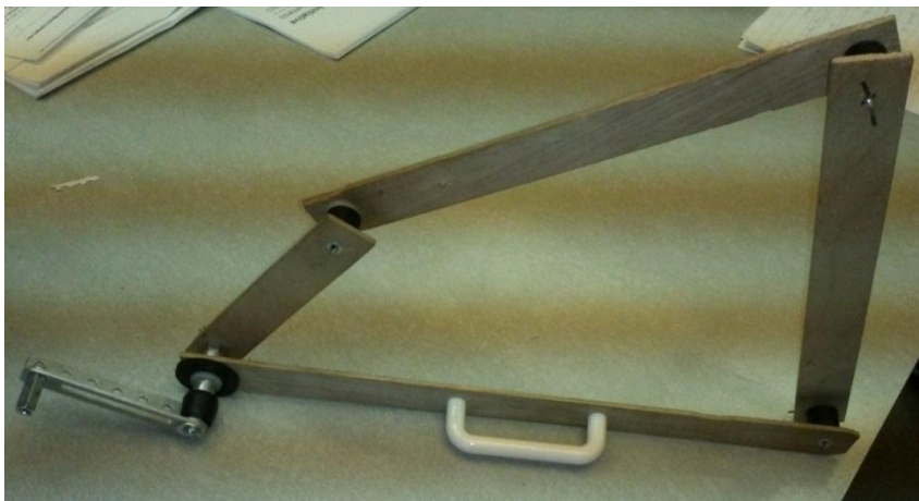
Figure 1, a system for constructing four bar pin jointed mechanism develop from scratch by one of the groups of students.
