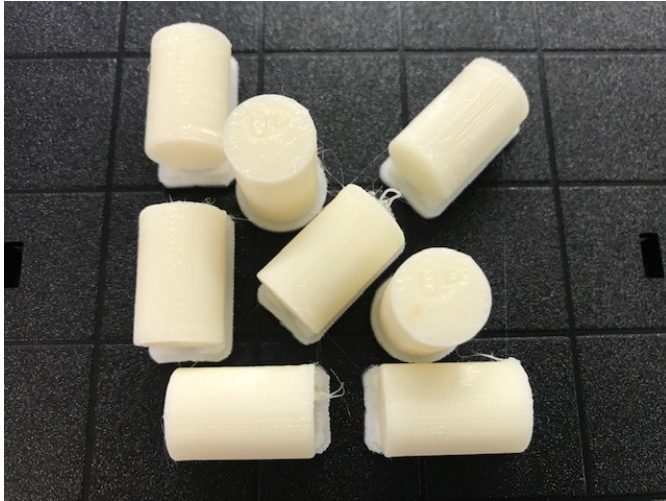
Figure 4. Orientations of Specimens at 3D Printing
