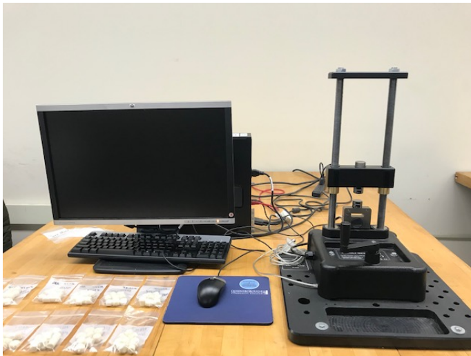
Figure 6. PASCO ME-8244 Comprehensive Materials Testing System
