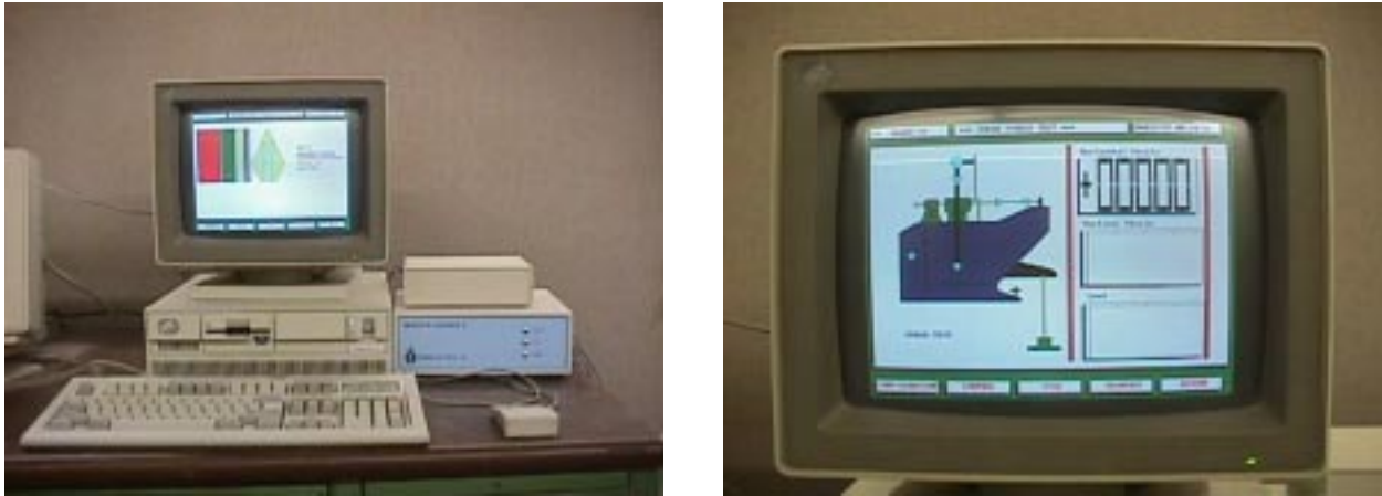
Figure 3. A) 386 Computer & Data Acquisition System B) Monitor Display of Direct Shear Test
