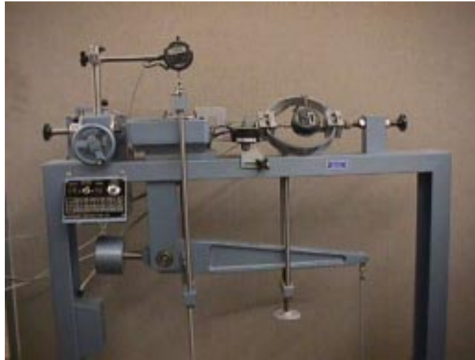
Figure 1. Photo of Typical Direct Shear Apparatus.
