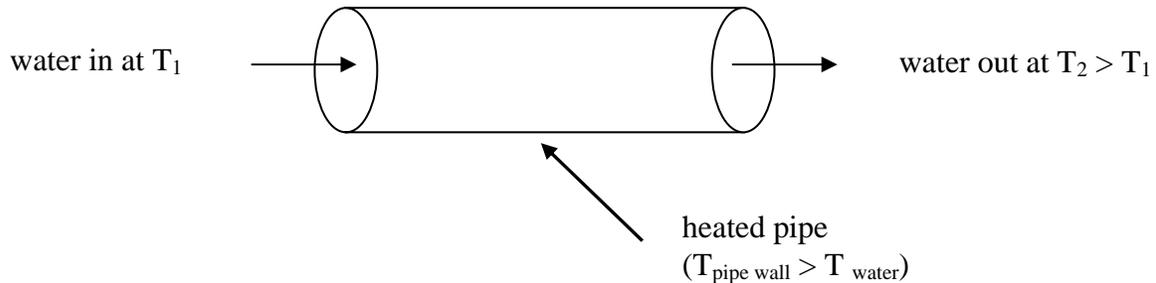
(Heatpipe1) If the pipe wall temperature and water velocity are constant, what can be said about the water flowing through the pipe:
