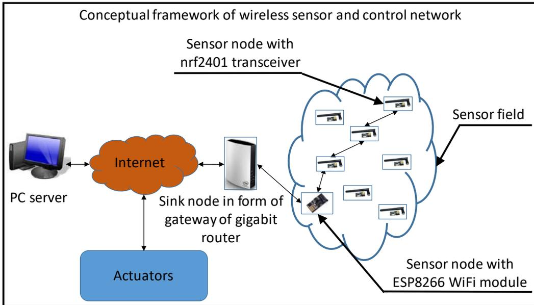
Figure 1: A PC server-based wireless sensor network topology
