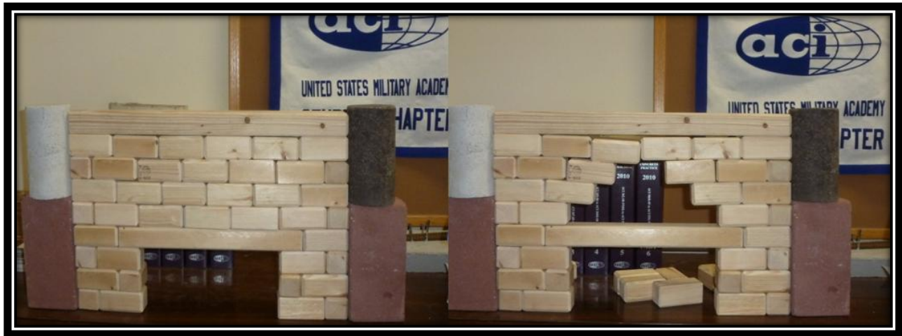
Fig. 8: A simple wall constructed of wood blocks provides a model of a masonry lintel and arch action
