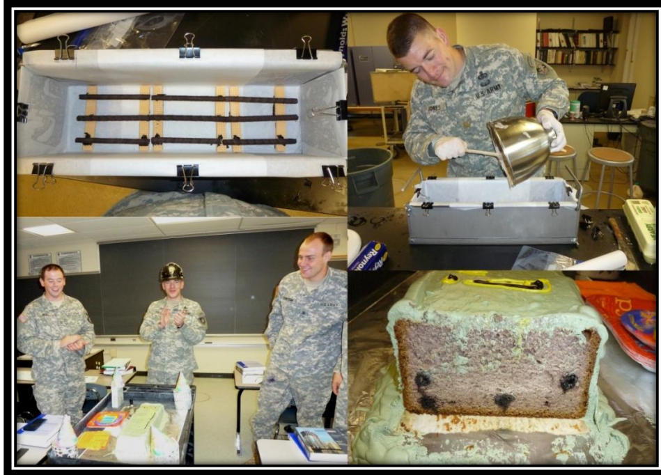
Fig. 2: The production of (and a look inside) a reinforced cake beam
