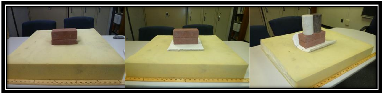
Fig. 4: A foam model provides demonstrations of the benefits (and failure modes) for a slab-on-ground
