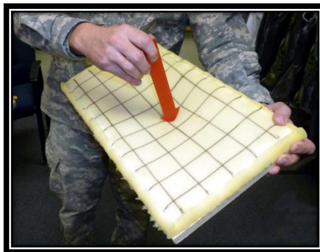
Fig. 3: A model of a one-way slab. The grid helps students visualize the large difference in the transverse and longitudinal curvatures
