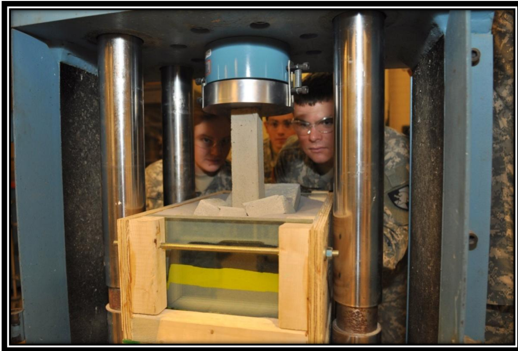
Fig. 7: A sandbox and universal testing machine can be used to demonstrate soil-structure interaction and failure modes of reinforced concrete footings
