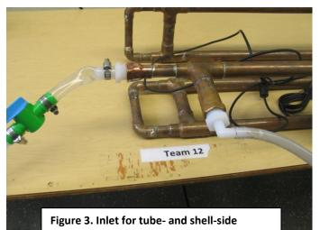
one of my past heat transfer classes). A "hot" process stream (tap water) flows from a reservoir (blue tank in the picture) equipped with a small submersible pump. The water flows through a manually controlled valve (green valve shown at left) and through the "tube side" (i.e. inner ½" copper tube) of the double-pipe heat exchanger. A cold stream (ice water) is fed to the "shell side" (i.e. a ¾" sealed copper tube) to cool the process stream to a specified temperature.
