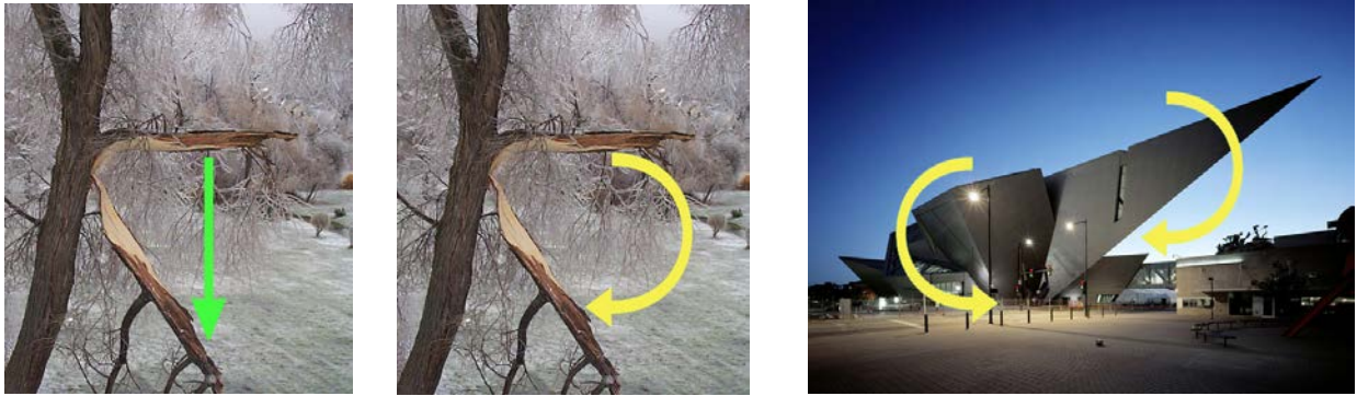
Figure 3-1 The students are instructed to view the limb as being “rotated” about the junction instead of falling “vertically” down. As a result, structural eyes to “read” the rotational equilibrium in architectural forms are properly developed.
