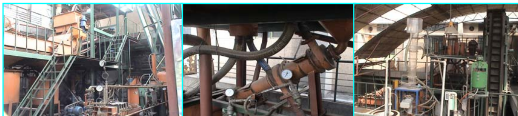
FIG 7 Pilot systems of dense medium separation and flotation of fine coal
