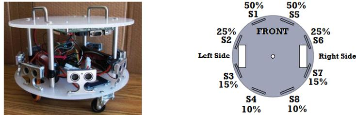
Figure 1. a) Mobile Robot Platform and b) Sonar Sensor Layout and Weights
