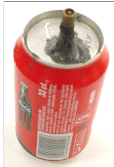
Figure 10 – Can prepared for dome reversal investigation
