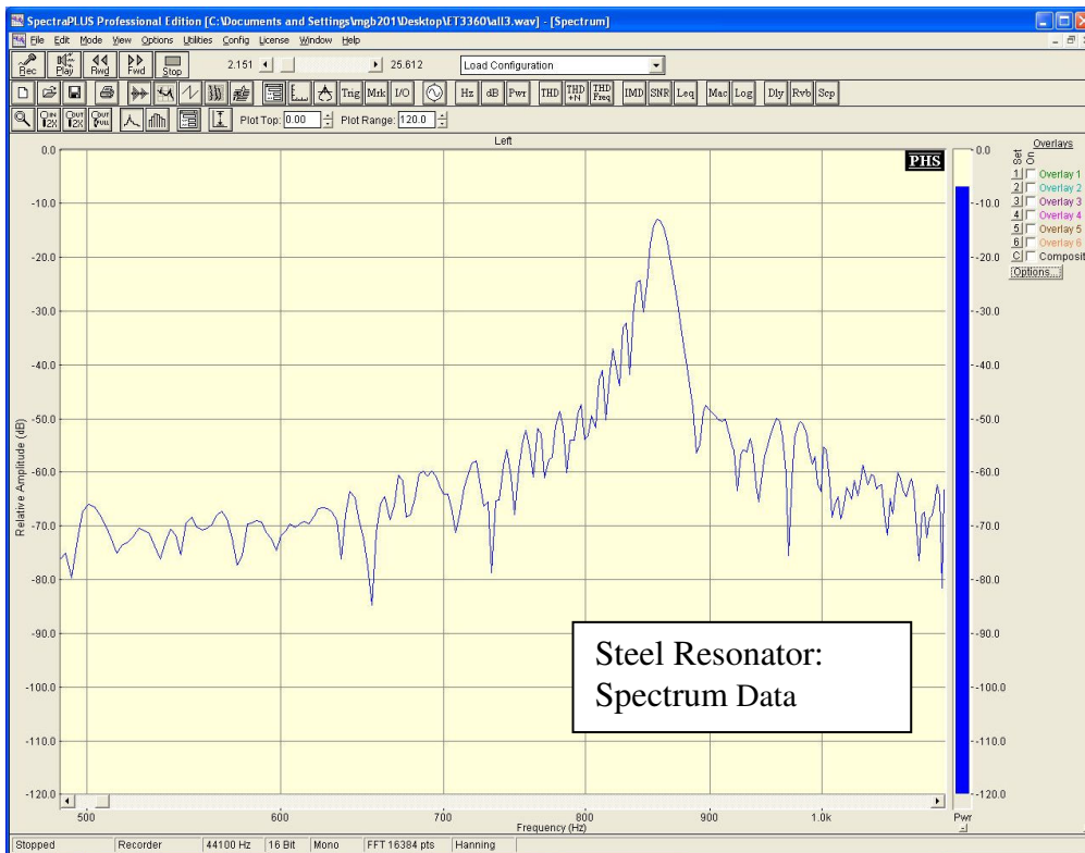
Figure 11. Helmholtz resonator frequency response (Team-2 data, fall of 2009).
