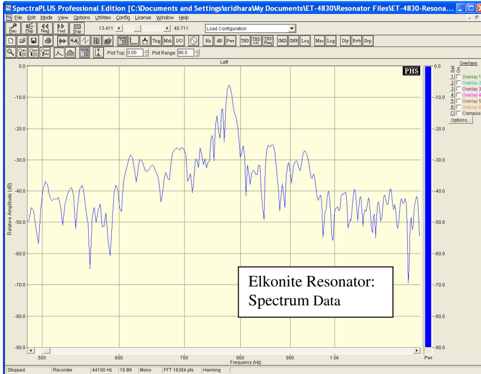
Figure 13. Helmholtz resonator frequency response (Team-1 data, fall of 2009).
