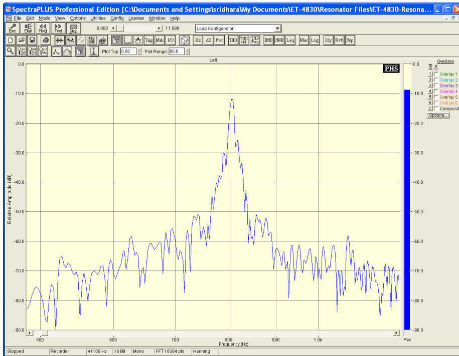
Figure 8. Helmholtz resonator frequency response (fall of 2008 data).
