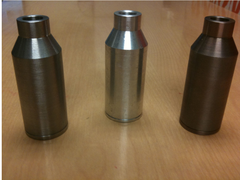
Figure 4. Steel, aluminum and Elkonite resonators designed and fabricated by Team-1 (Fall of 2009).
