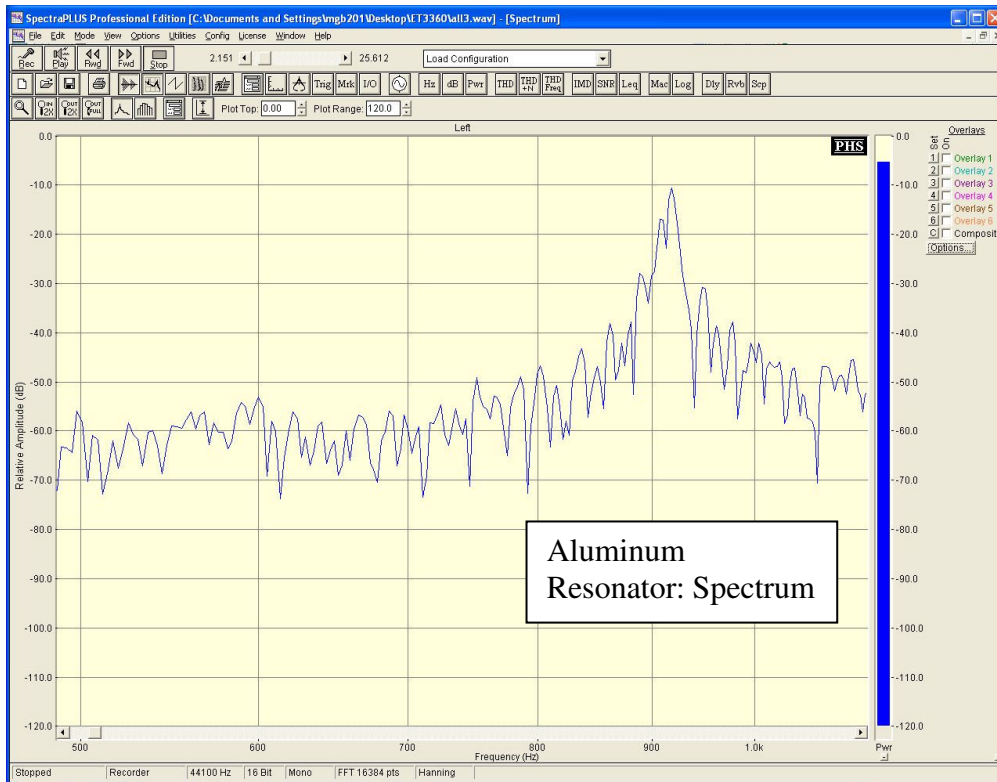
Figure 10. Helmholtz resonator frequency response (Team-2 data, fall of 2009).
