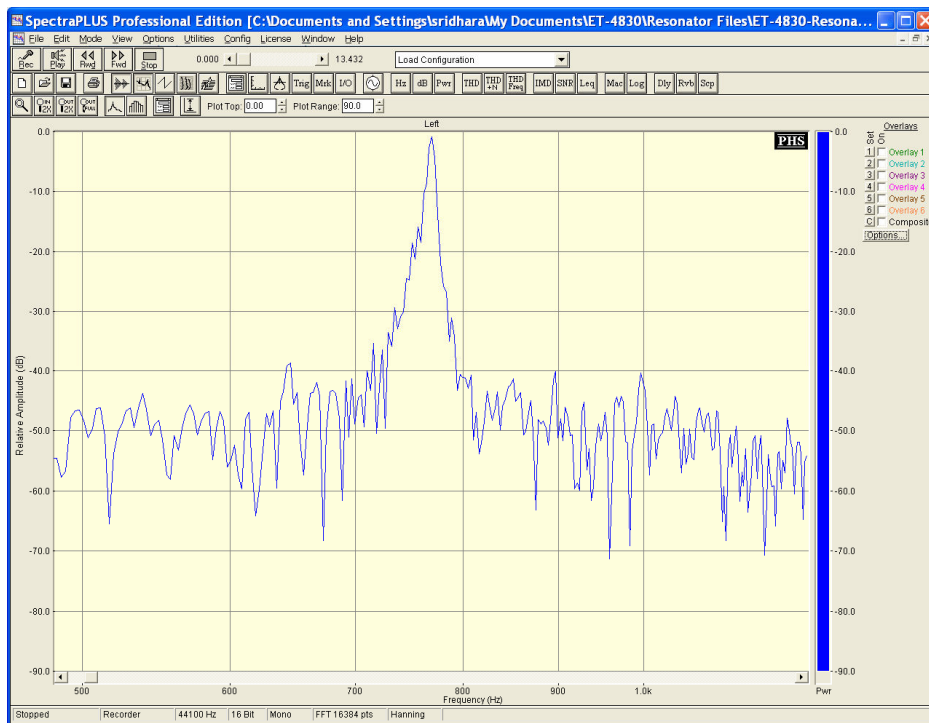
Figure 7. Helmholtz resonator frequency response (fall of 2007 data).
