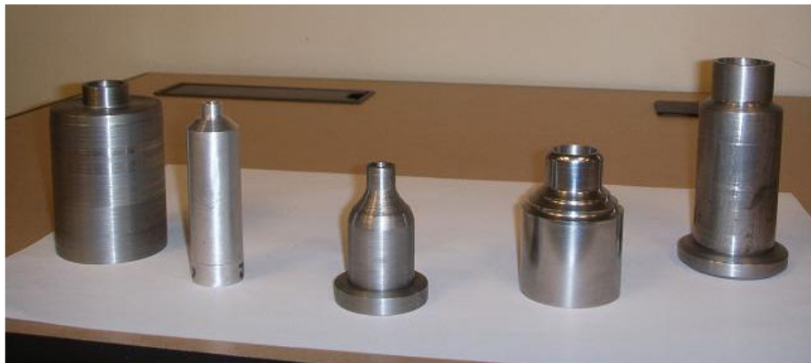
Figure 3. Steel and aluminum Helmholtz resonators built by student teams and the author.
