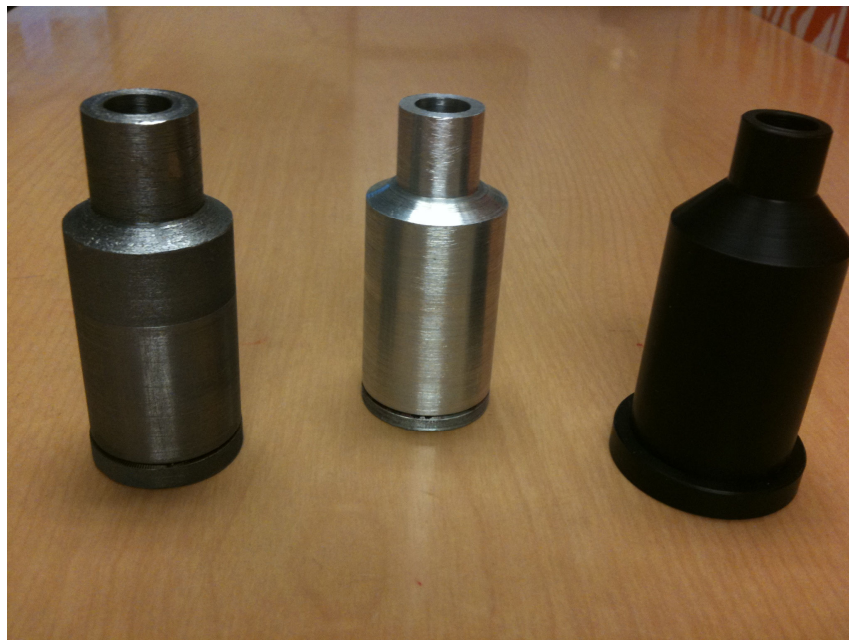
Figure 5. Steel, aluminum and Delrin resonators designed and fabricated by Team-2 (Fall of 2009).
