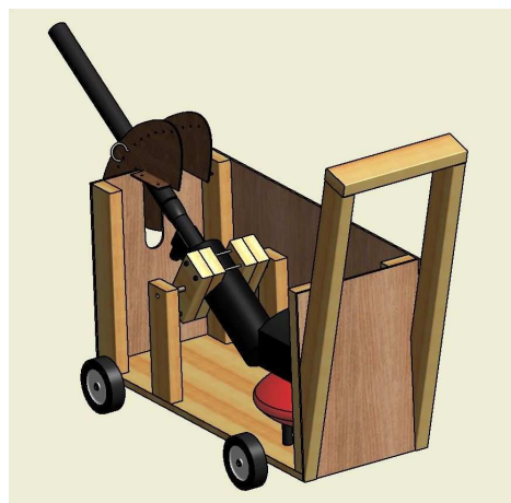
Figure 7. Isometric view of the golf ball shooter created using AutoDesk Inventor
