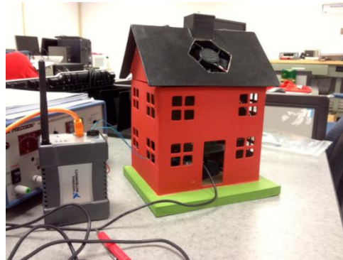
Figure 6 mySmart: smart home monitoring and control
