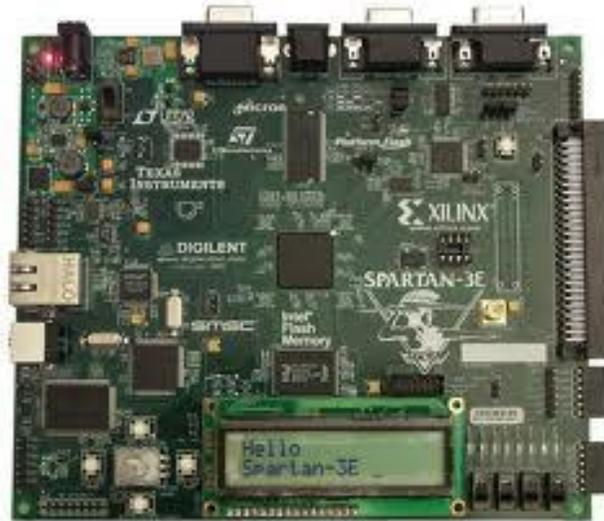
**Figure 4.** FPGA board used for lab experiments in ECE 238 Computer Logic Design.
