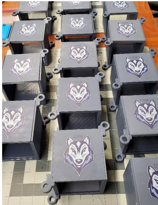
Figure 1: 3-D printed 1U CubeSat chassis provided to competition registrants. Corner rings provided as high-altitude balloon attachments. Photograph courtesy of So Young Han.
