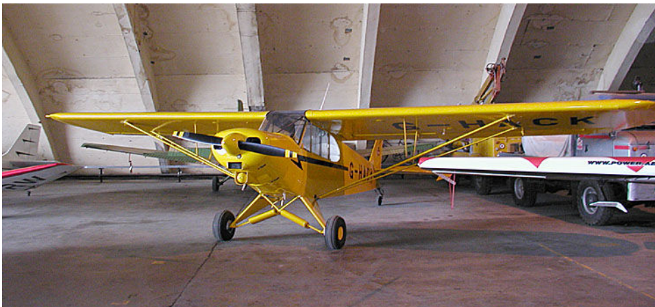
Figure 3 - Aircraft with a Tail Dragger Landing Gear Taken from the Public Domain at http://en.wikipedia.org/wiki/Image:Piper.cub.750pix.jpg .
