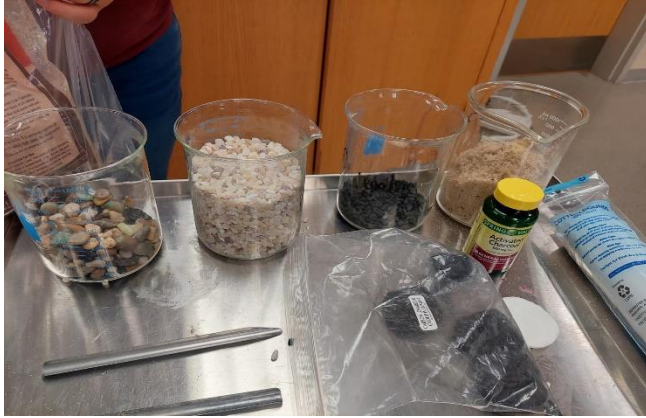
Figure 5: Materials for simulating wastewater treatment processes: sedimentation, filtration and biological treatment
