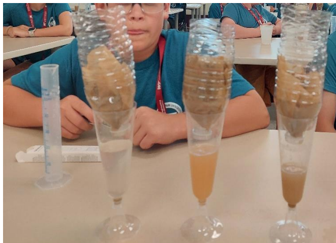
Figure 3: Demonstration of porosity and permeability using recycled bottle filters with varying sediment layers.
