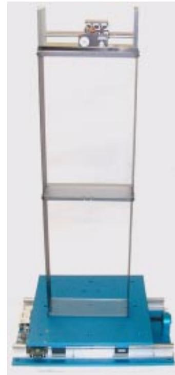
**Figure 1. Bench-Scale Shake Table with Model Building and Active Mass Driver.**
