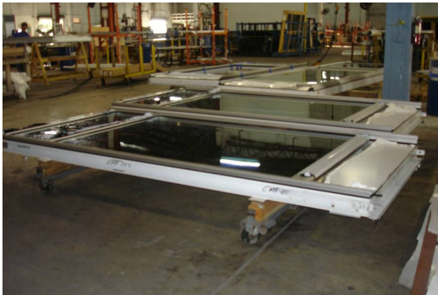
Figure 1: Unitized curtain wall
