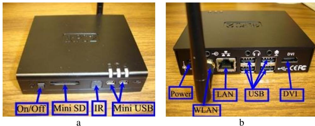
Figure 3. Fit-PC2, front (a) and back (b)
