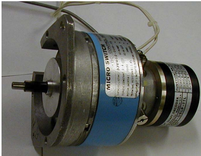
Figure 9. DC Motor and Shaft Encoder
