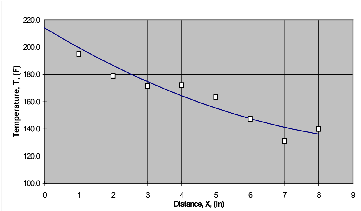
Figure 13: Conical Fin, Average
