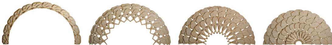
Fig. 2 Folding sequence of Hoberman arch [5]
