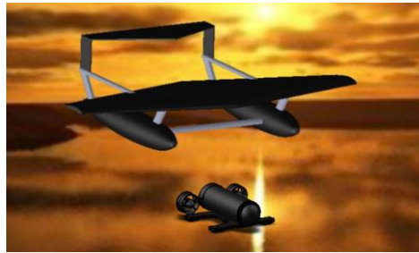
Figure 2. Schematic view of Titan-based fixed-wing drone.
