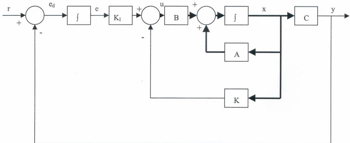
Figure 8: Block Diagram of Plant and State Feedback with Integral Control
