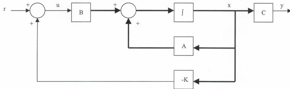
Figure 6: Plant with State Feedback
