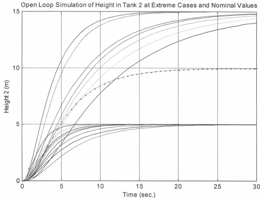
Figure 2: Responses of an open-loop system for a unit-step input for 16 extreme cases
