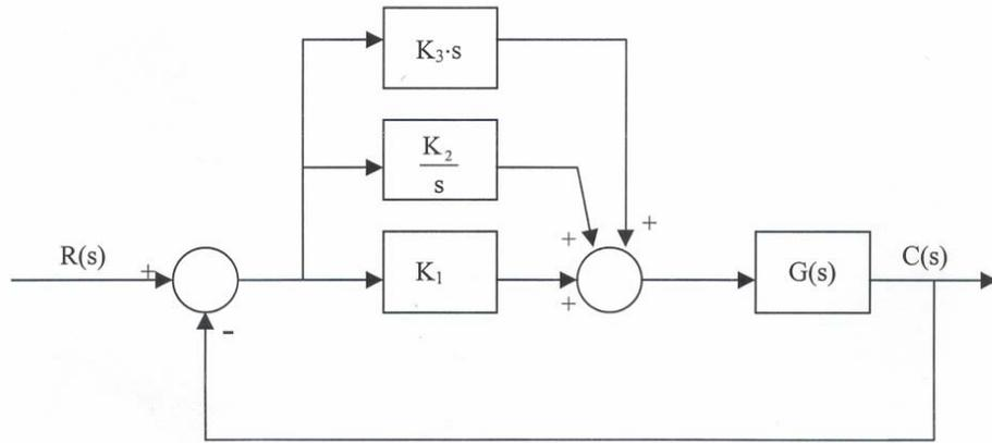
Figure 4: Closed-loop system block diagram with PID Controller
