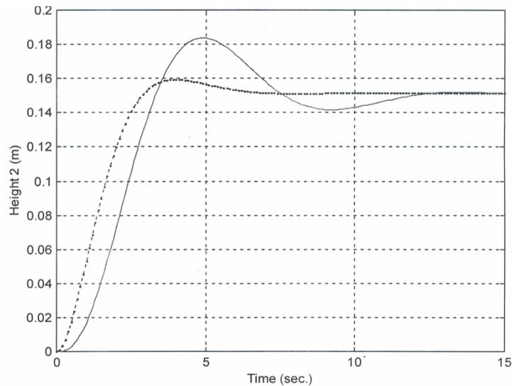
Figure 3: Height in Tank 2 using a PD-Controller
