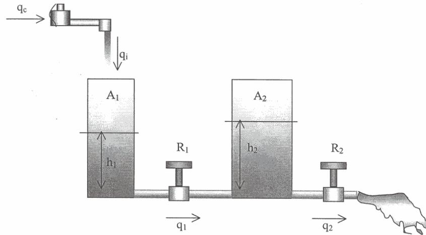
Figure 1: A two-tank liquid-level system.
