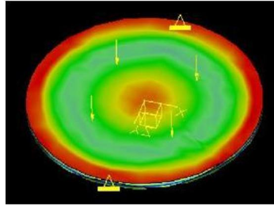
Figure 5: Contour plot of the von Mises stress in a circular membrane under a uniform applied pressure.
