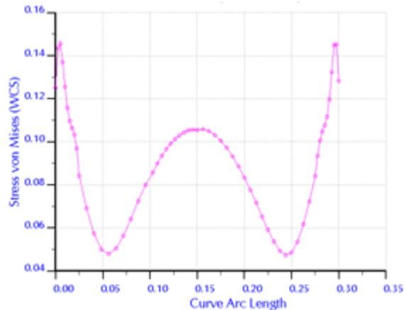
Figure 4: Graph of the von Mises stress across a diameter of a circular membrane subjected to a uniform applied pressure.
