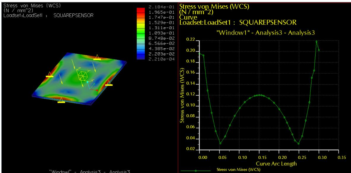
Figure 4: FEA results of square diaphragm subjected to a uniform pressure load.
