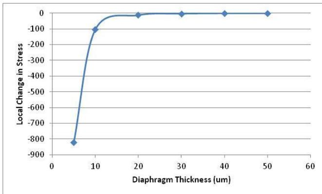
Figure 3: Localized change in stress as a function diaphragm thickness
