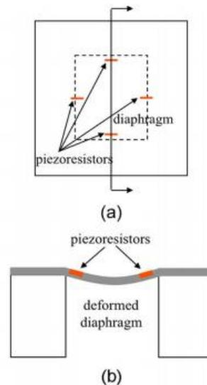
Figure 1 Example of a pressure sensor with piezoresistors oriented in both the transverse and longitudinal directions from (a) top and (b) section views [4].
