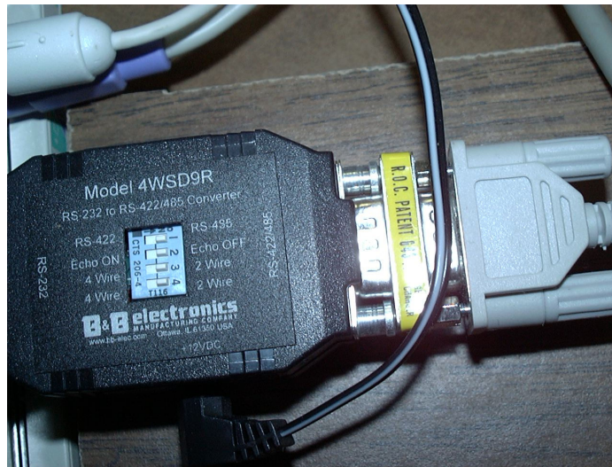
Figure 6. RS-232 to RS 422/485 Data Converter hooked up to the serial port of a PC.
