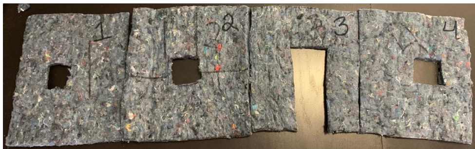
Figure 6. The insulation chosen and it cut into panels for the model. Pieces are labeled for each one has a different weight and volume.
